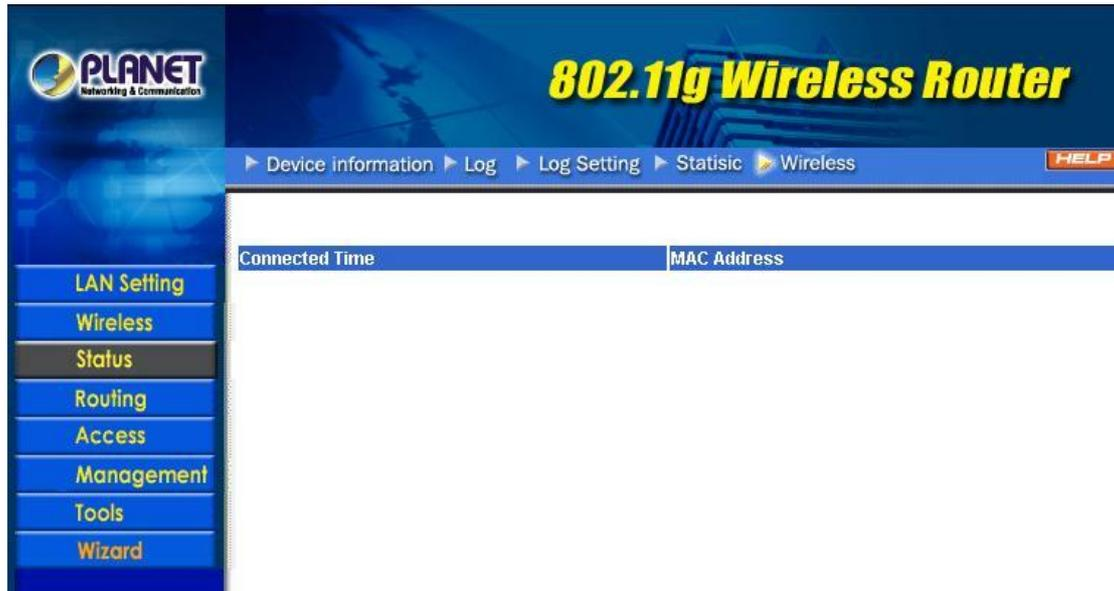
**Connected Time:** Displays how long the wireless device has been connected to the LAN via the WRT-410.
